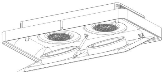
Open the bottom plate by pulling it open on the front side with 2 hands in a downward movement.
